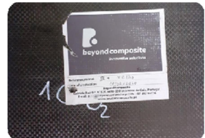
Composite panel after shot Back face
